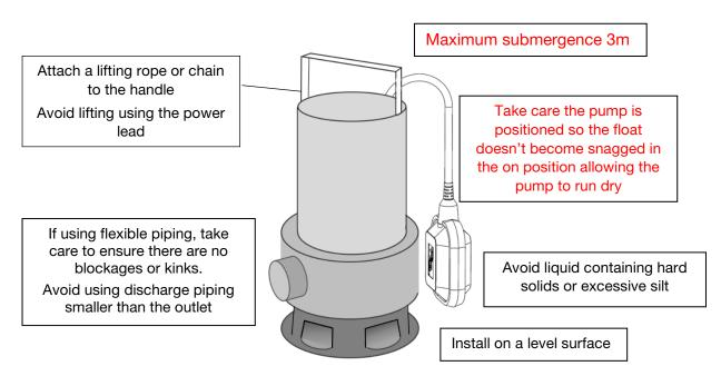
The pump should be connected to (10 amp) power and a <u>residual current</u> <u>device</u> or RCD with a nominal trip current installed in compliance with the requirements of AS/NZ 3000.
