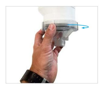
6 - Attach the Electronic Release Valve by first installing the 25mm x 20mm (1" x 3/4") reducing adaptor and washer to the 25mm (1") thread of the screw cap.
