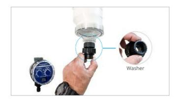
8 - Attach the valve at the union and orientate dial for easy access.
