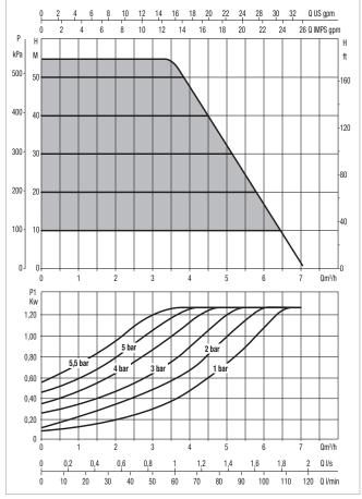
The performance curves are based on kinematic viscosity values  $= 1 \text{ mm}^2/\text{s}$  and density equivalent to 1000 kg/m³. Curve tolerance according to ISO 9906.
